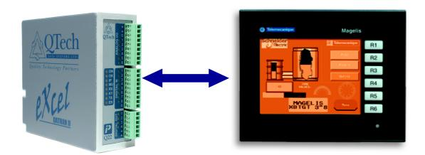
The Magelis HMI (Human Machine Interface) is a class leading 'touch screen' operator panel that can now be integrated with a DATRAN RTU to provide unprecedented clarity and real time visibility of plant operation.
